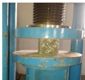
Fig 5. Cube Testing in CTM for trial 1 and 2 cubes
