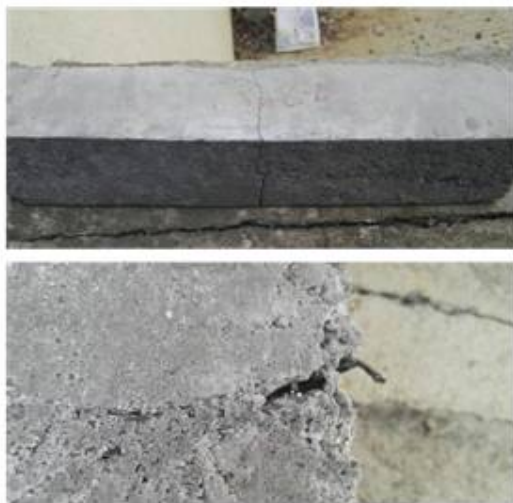
Fig.13. Placement of Geogrid in the tested sample
