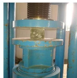
Fig 5. Cube Testing in CTM for trial 1 and 2 cubes
